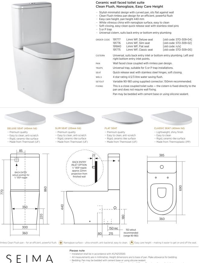
Fix pan to floor using a sand cement mixture of 3:1 to a depth of 60mm. Do not use lime or fast-drying cement. - Bracket fixing: The pan should be bedded with silicone sealant and fixed with the brackets supplied.
